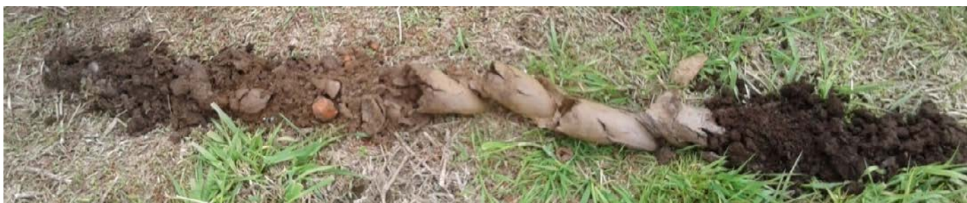
Soil profile in Zwolle, from left to right: Topsoil, mixed soil with sand, clay layer, peat
